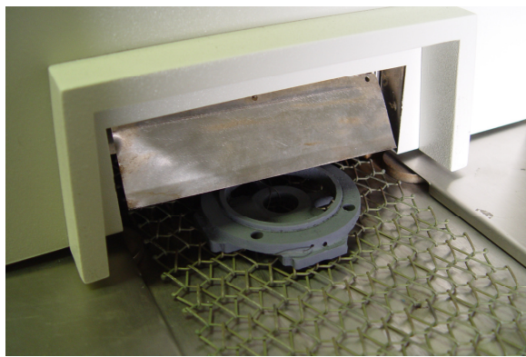
Figure 9-11 Brass forging sample exiting furnace
