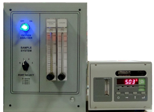
Figure 3-2 Sample System Console & Oxygen Analyzer
