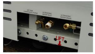
Figure 2-35 UCD Water Connections and Air Purge (Reservoir option only)
