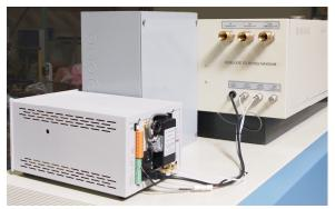
Figure 2-31 Locate oxygen analyzer next to OSS
