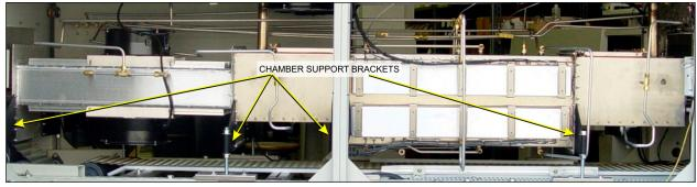
Figure 2-7 Location of Support Brackets on post-2000 model furnaces
