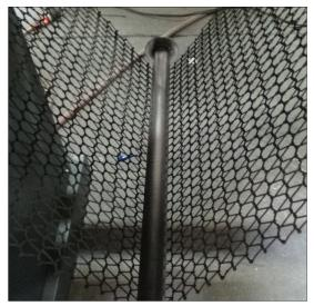
Figure 2-15 Proper Alignment of Belt Weight
