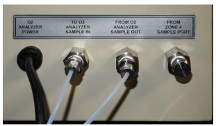
Figure 2-33 OA furnace control enclosure connections
