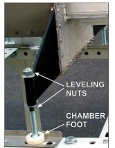
Figure 2-5 Chamber Support Bracket
