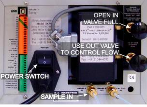
Figure 2-34 EC913 Oxygen Analyzer Rear Controls
