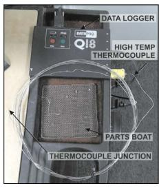
Figure 9-5 Temperature Profiling Apparatus
