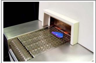
Figure 9-9 Silicon Wafer Entering Furnace
