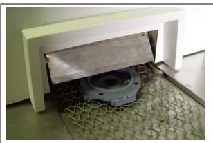
Figure 9-11 Brass forging sample exiting furnace
