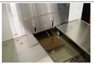
Figure 9-12 Sample plate exiting furnace
