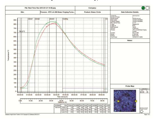
Figure 9-14 880 °C Brass Forging profile
