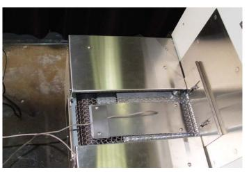
Figure 9-8 Metal Plate Sample with Wire Sheath Type K Thermocouple
