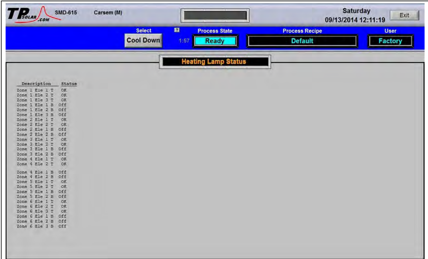
Figure 3-24 Lamp String Failure screen
