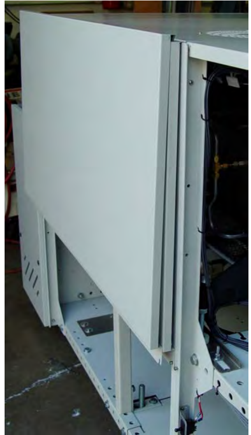
Figure 3-6 Hanging Lower Access Panel
