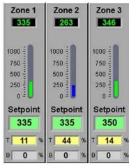
Figure 2-10 Zone Temperature display
