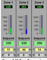
Figure 2-25 Zone Temperature & Power setpoints
