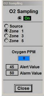
Figure 2-31 O<sub>2</sub> Sampling display and Port Select
