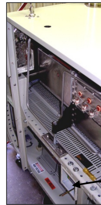
Figure 1-16 Typical safety interlock disconnect switch location (option)
