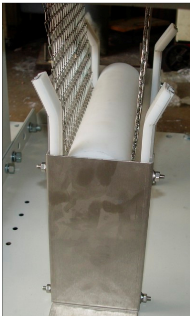
Figure 1-12 Belt Weight in Place
