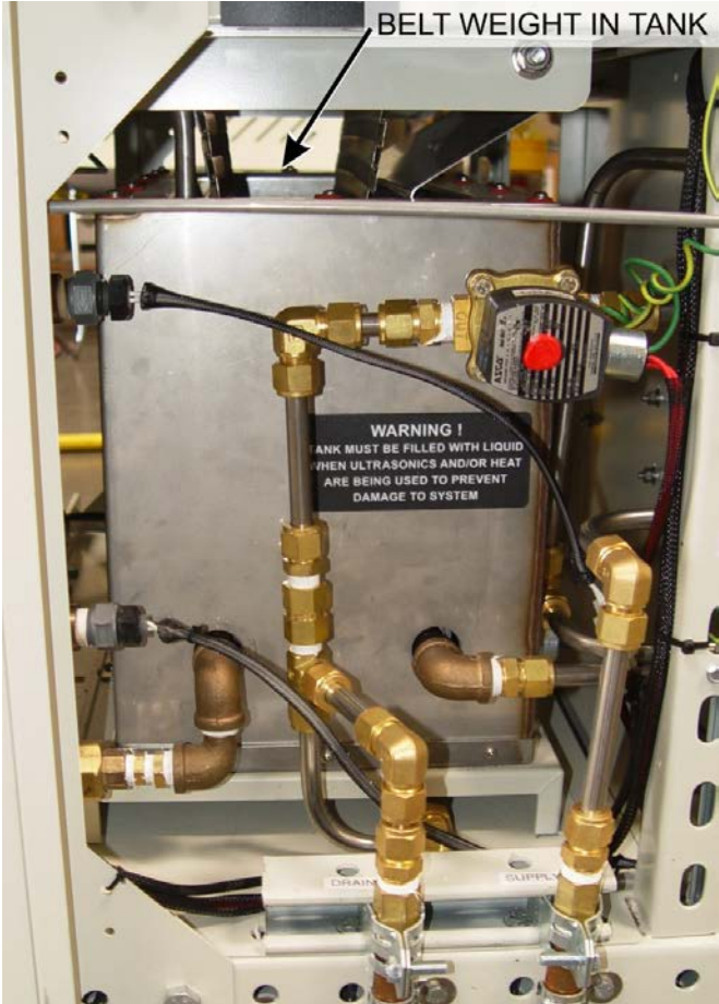
Figure 1-14 Belt weight in Tank on UCD system
