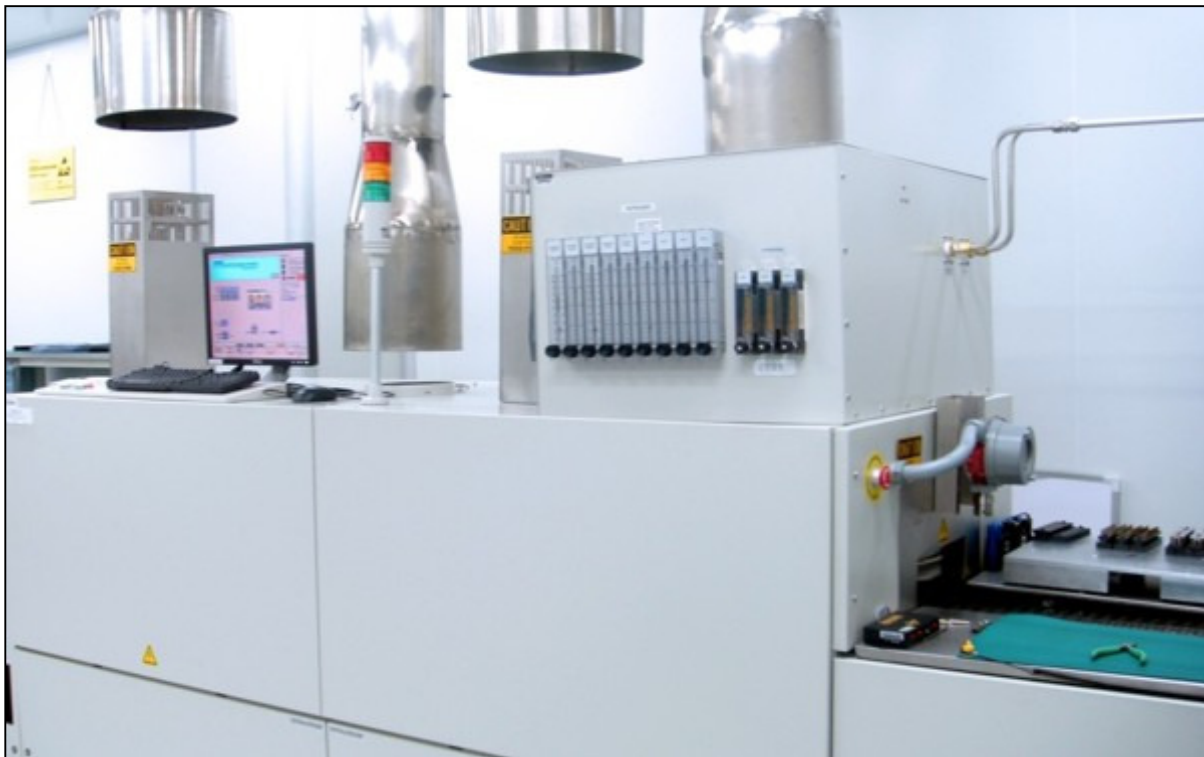
Figure 1-35 Typical Hydrogen Furnace Process Gas Exhaust Connection
