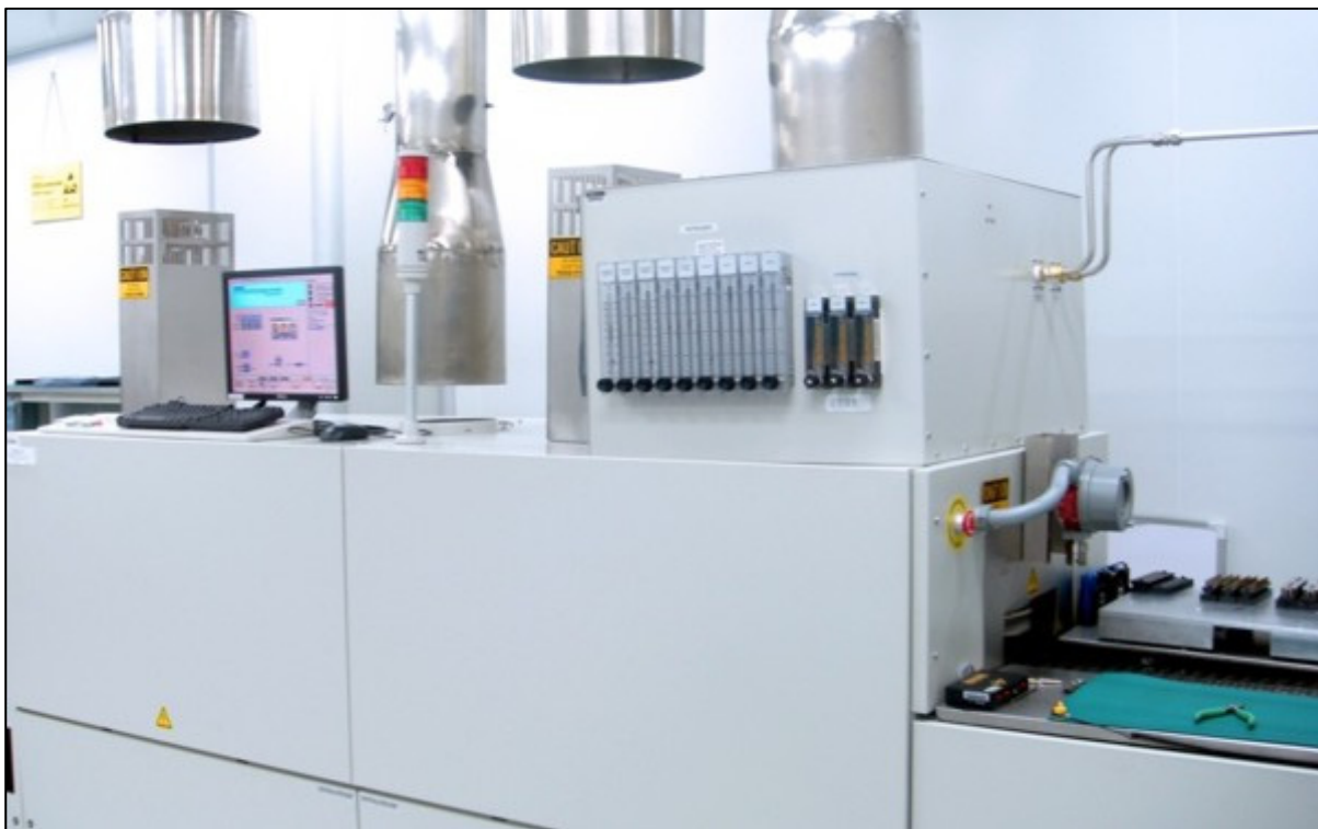
Figure 1-35 Typical Hydrogen Furnace Process Gas Exhaust Connection
