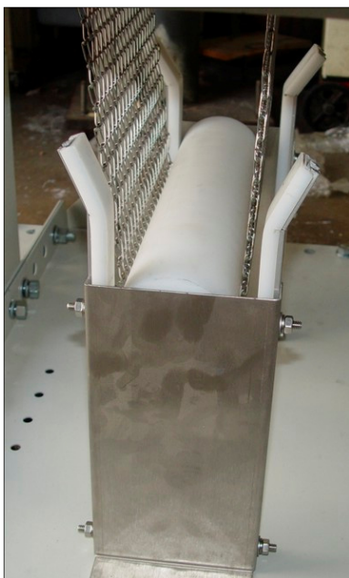
Figure 1-12 Belt Weight in Place
