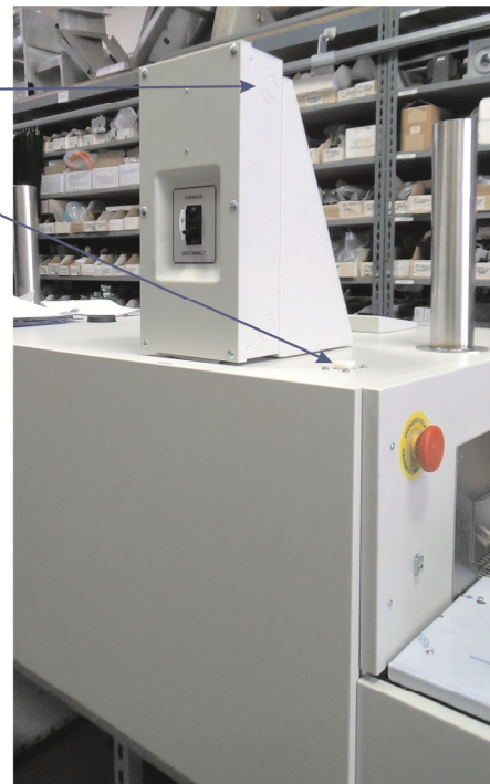
Figure 1-17 Typical circuit breaker enclosure location (option)
