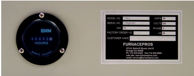
Figure 1-16 Elapsed Time Meter and Nameplate
