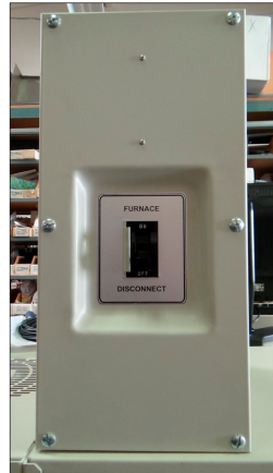
Figure 1-18 Circuit Breaker enclosure
