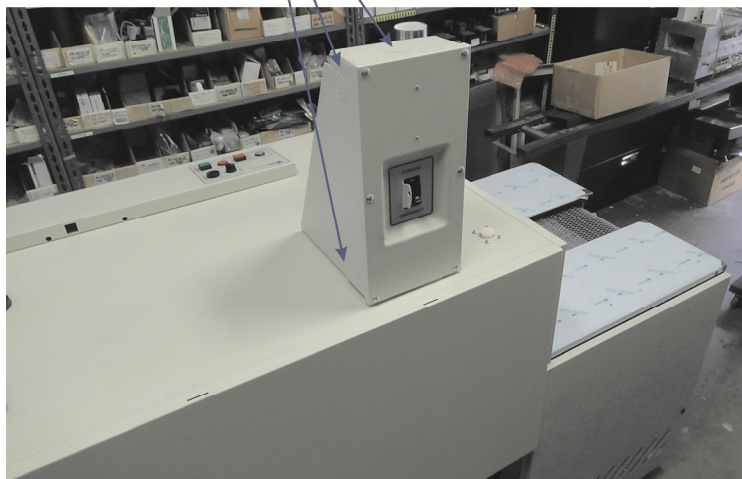
Figure 1-17 Typical circuit breaker enclosure location (option)
