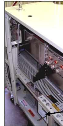
Figure 1-15 Typical safety interlock disconnect switch location (option)
