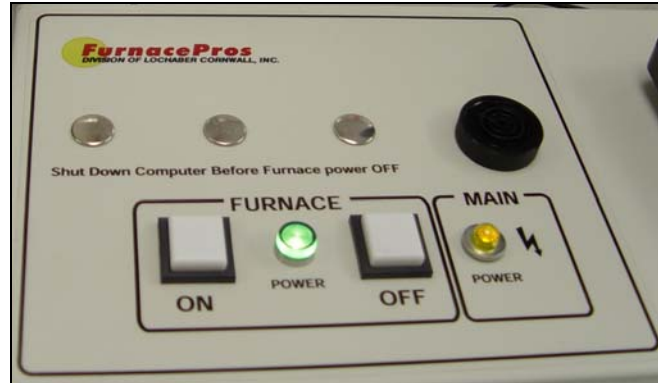
Figure 2.4.1 FURNACE ON and FURNACE OFF buttons
