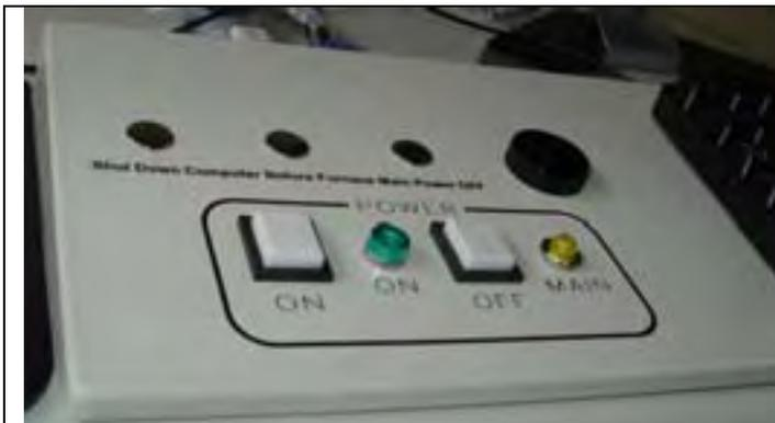
Figure 2.1.1 Control Panel showing POWER ON and OFF and Indicator Lights
