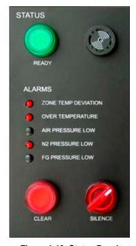
Figure 1-19 Status Panel and Alarm Controls
