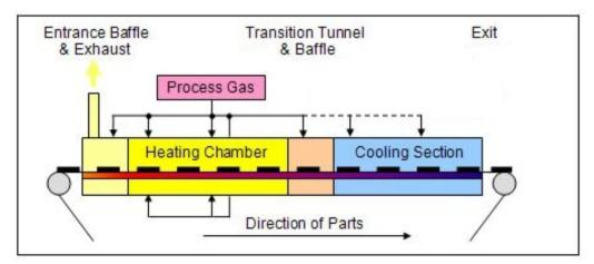
Figure 1-8 Process Sections
