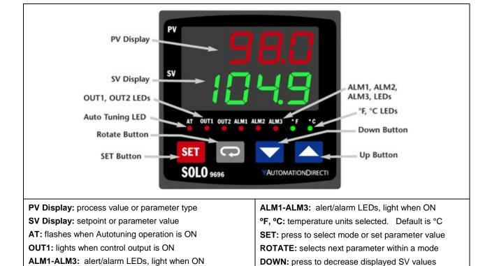
Figure 1-14 Temperature Controller Indicators and Control Buttons
