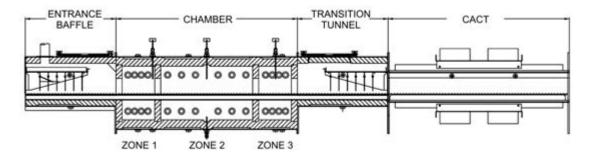
Figure 1-9 Furnace Internals
