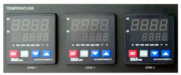
Figure 1-13 Zone Temperature Controllers
