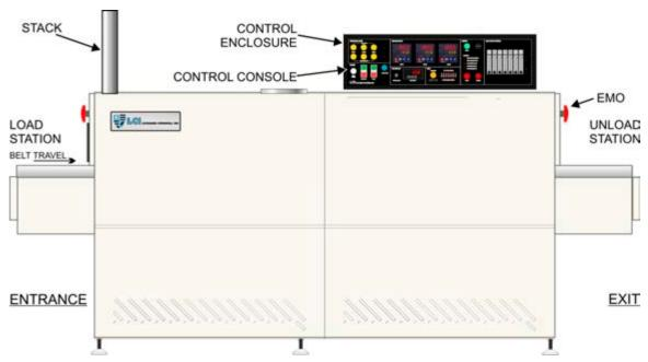
Figure 1-1 Furnace Front Elevation
