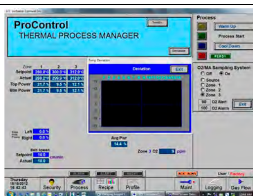
Figure 0-13 O2 ppmv on Process screen
