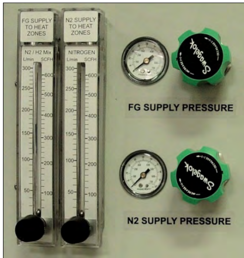
Figure 0-15 Controls for Supply Gas Mixing System. (Only available on Dual Gas Furnaces)
